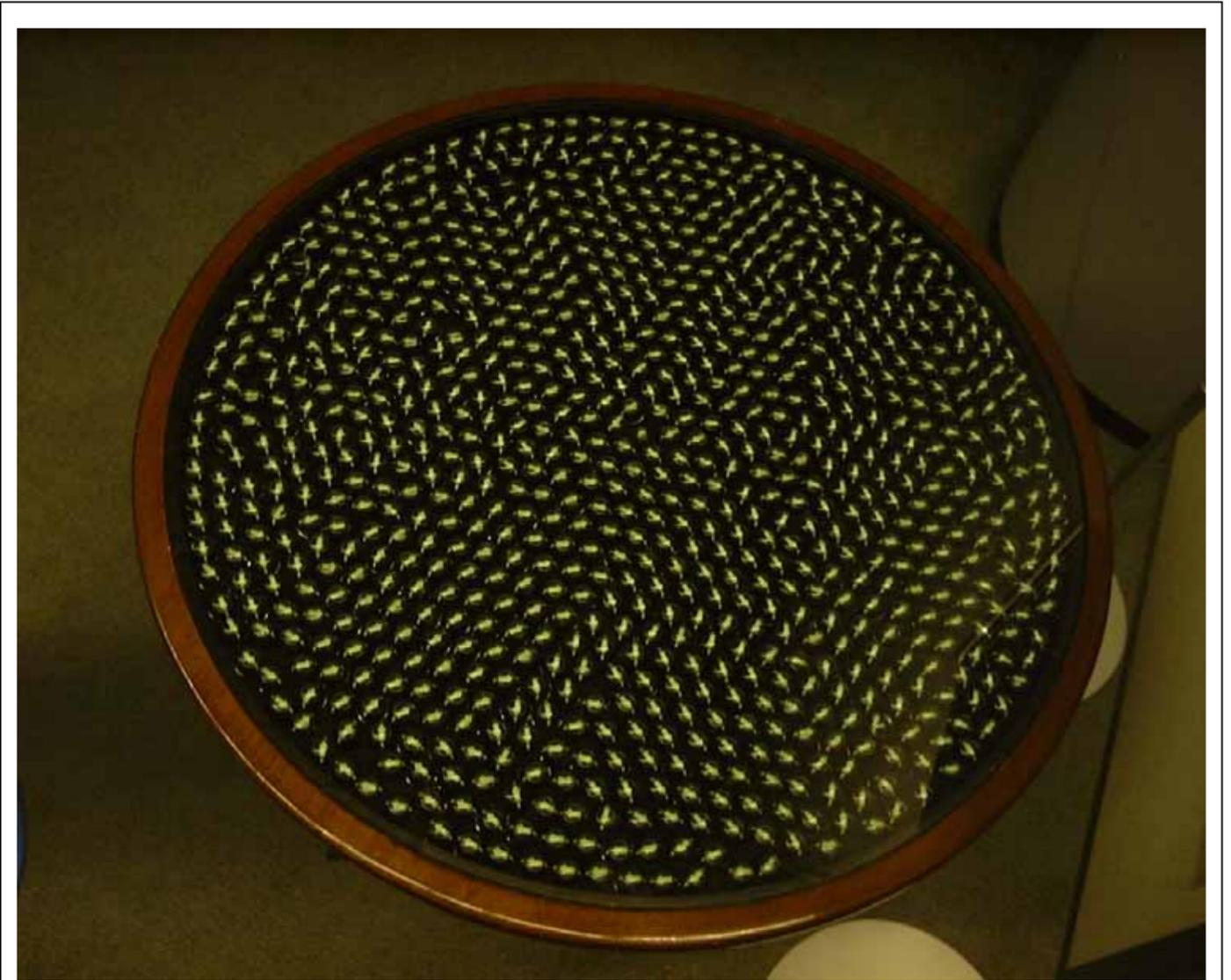
Fig.2 Magnetic domains on a crystal of 1000 magnetic compasses
