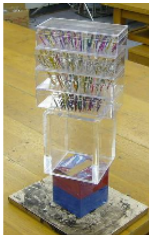
Figure 3. Demonstration of magnetic field lines. Iron wires in transparent acrylic cases show magnetic field lines coming out of a cubic magnet with the edge length of 100 mm. The magnetic flux density of the magnet is about 0.5 T at the surface.
