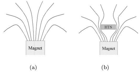
FIG. 5: Diagram of the Meissner effect. (a) The free magnetic field lines diverging from a magnet. (b) The magnetic field lines are excluded from the HTS (Meissner effect).
