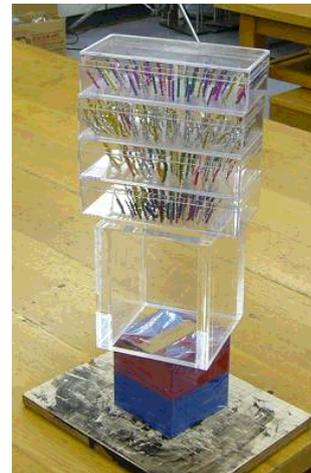
FIG. 3: Magnetic field lines diverging from a 100mm cubic NdFeB sintered magnet of magnetic flux density about 0.5T at the surface. The magnetic field lines are shown by the iron wires in the acrylic cases.
