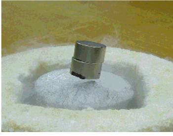
FIG. 11: Rigid levitation of a NdFeB sintered columnar magnet above a superconductor.
