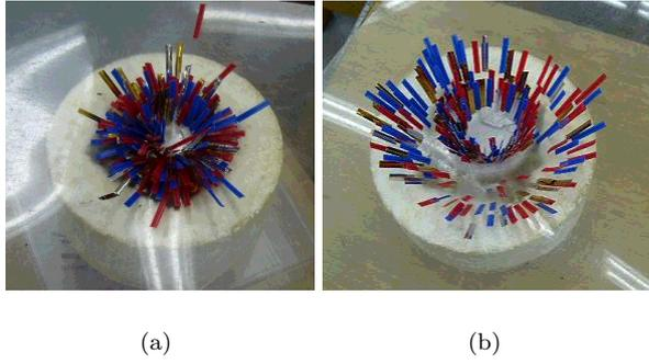
FIG. 7: Pinning effect against increasing external magnetic field strength. The magnetic field lines diverging from NdFeB sintered ring magnet are “copied” into the HTS. The HTS is at a distance of (a)190mm, (b)60mm, from the 100mm cubic NdFeB sintered magnet. There are the wires on a transparent plastic board on the top of the HTS. It is shown by the wires that the magnetic field lines penetrate a ring area in the HTS and do not move in it for the change of the external magnetic field strength.
