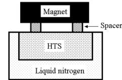
FIG. 6: A cooling method to cause Fig. 2. Before cooling, the magnetic field lines of the magnet penetrate the HTS, and after cooling, they are pinned in the HTS.
