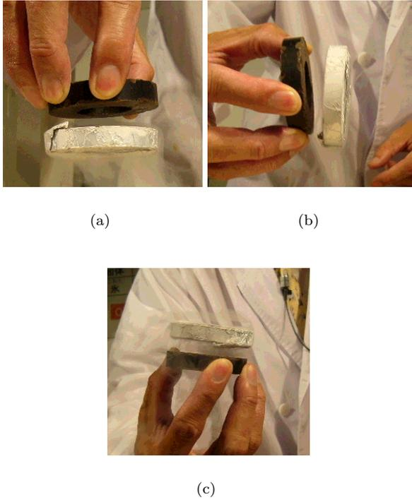
FIG. 2: Superconductor bound by a magnet at a fixed distance. (a) A HTS is suspended by an NdFeB sintered ring magnet (the held black object). (b) (c) The magnet is cap-sized. The relative position of the HTS and the magnet is kept at a fixed distance.
